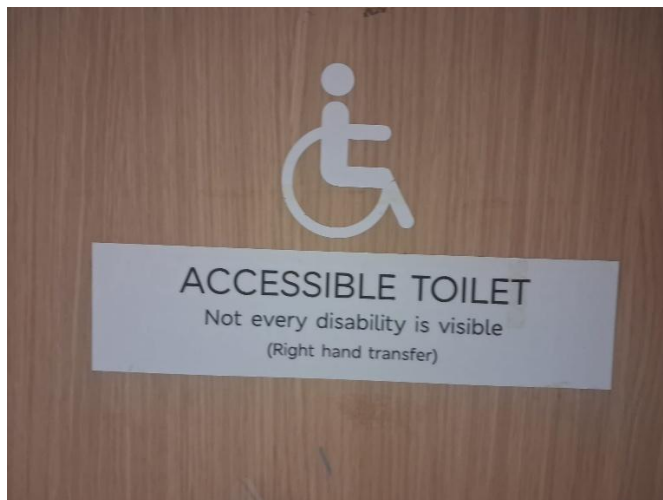
Figure 7: Toilet door sign indicating transfer side
